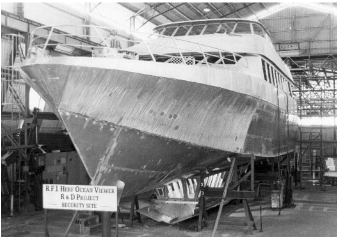
1.2 A Richardson and Associates (Australia) Ocean Viewer all-aluminium vessel. The hull is 5mm thick A5083. Courtesy TWI Ltd.
